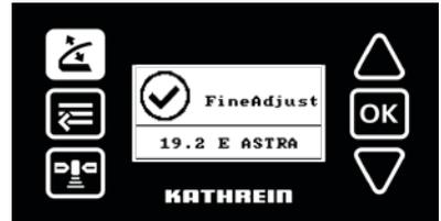
⇒ The display on the right is shown after a successful satellite search. The found satellite, the signal strength and the signal quality are displayed.
