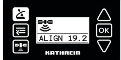
⇒ After the satellite has been found, a fine adjustment of the antenna is carried out. The display shows the image on the right.
