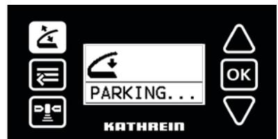
⇒ When the antenna is in the park position, the display on the right is shown.
